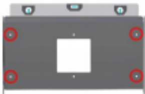
Step 1 Mark drill holes
